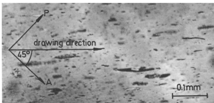
Fig.1. Micrograph of PE drawn film, immersed in silicon oil, taken at crossed polarizers.
